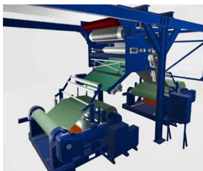
Dual wind-up with cutting system for automatic bobbins' change
